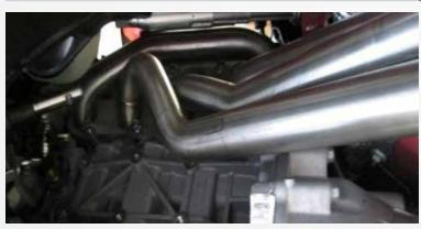
Install the supplied gasket and the BBK Header on the remaining studs and install the nuts and bolts. You may have to raise or lower the motor a bit to get the BBK header in place tighten all the nuts and bolts that you can reach from underneath the vehicle.
