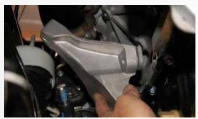
Utilizing a jacking device and a block of wood under the bell housing, remove the previously loosened nut on the driver side motor mount, once removed jack the engine upward enough to clear the motor mount stud. Remove the 4 bolts that secure the aluminum mount to the engine block and remove from the vehicle.
