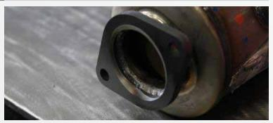
Remove the catted down pipe from the vehicle and fully weld the inside of the flange to the inside of the catted down pipe .
