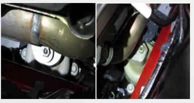
Remove the air filter box. Remove the first and second nuts on the top row of studs on the stock header of the driver side. On the passenger side, remove the first top nut that is behind the AC hose. Loosen the motor mount nut that faces up towards the header on each side, however do not remove completely at this time
