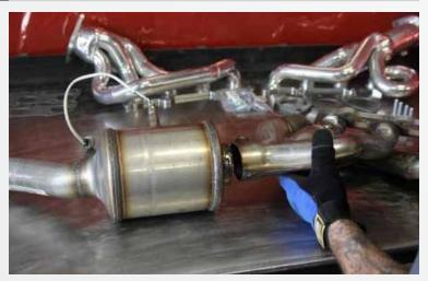
Using a Saws All or band saw cut on the weld that joins the stock exhaust manifold to the catted down pipe as shown in the pictures below.
