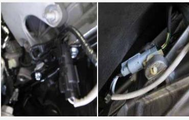
Lift the vehicle as high as possible utilizing approved jack stands or preferably a vehicle hoist. From underneath the vehicle unplug the 4 oxygen sensors from the wiring harness.
