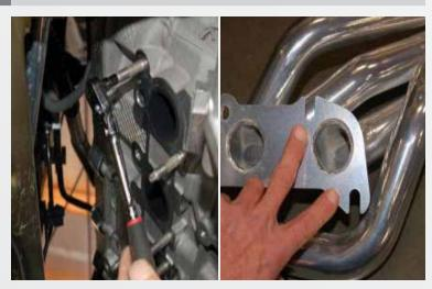
Using an 8mm Torx Bit socket remove all the exhaust manifold studs from the engine block except for the ones that correspond to the (2) notches in the BBK header flange that are closest to the firewall.
