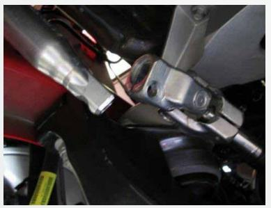
Remove the 2 bolts from the steering U-joint at the rack and pinion. Then pull the coupler downward towards the rack and pinion to separate the steering shaft from the coupler allowing the steering shaft to hang out of the way to the side.
